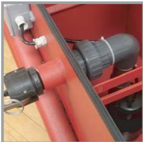
Return pump allows liquid return at 38 gallons/minute.
