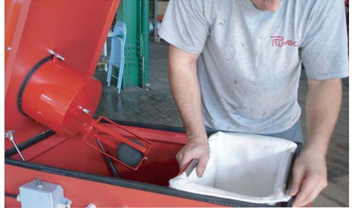
Designed to collect liquids and solids, separate the solids, and return the liquids for reuse.
